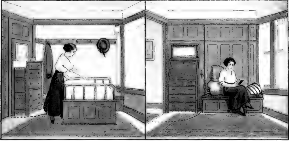
The Heavy Door Has a Chiffonier on One Side and a Desk on the Other. The Bed Can Be Folded Up to Form a Seat. Thus a Comfortable Bedroom Can Be Transformed into a Cozy Sun-Parlor
